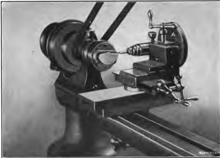
Fig. 10. Milling Attachment for Bench Lathe used for Milling Small Punches, Dies, etc.
