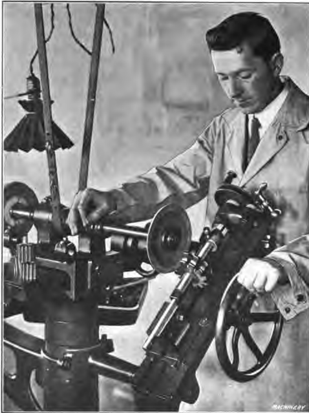
Fig. 11. Grinding Form Cutters by Means of a Form Cutter Grinding Attachment
