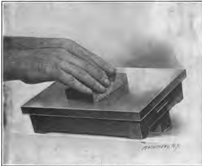
Fig. 6. Charging a Flat Lap, using a Hardened Steel Block
