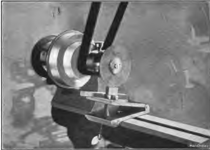
Fig. 13. Adjustable Plate for Surface Grinding on the Bench Lathe
