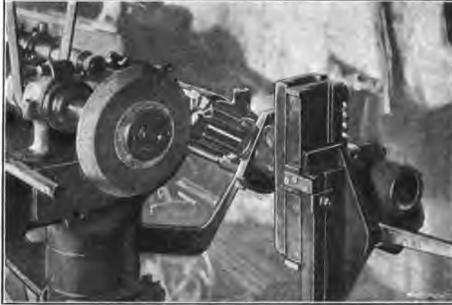
Fig. 19. Grinding End-mill Teeth to Shape
