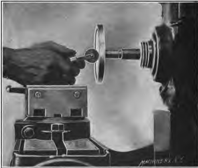
Fig. 8. Charging the Lap with a Roller
