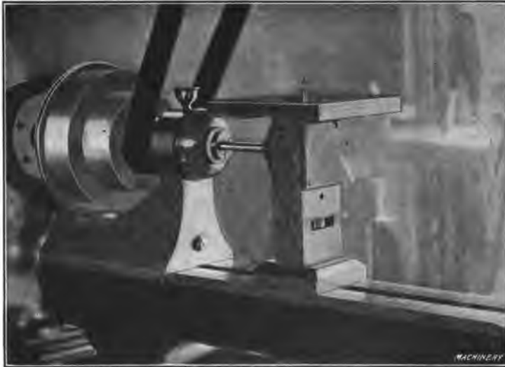
Fig. 11. Vertical Milling Attachment for Machining Die Stripper Plates, etc.
