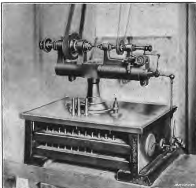
Fig. 14. Lapping a Small Chuck or Collet in Bench Lathe
