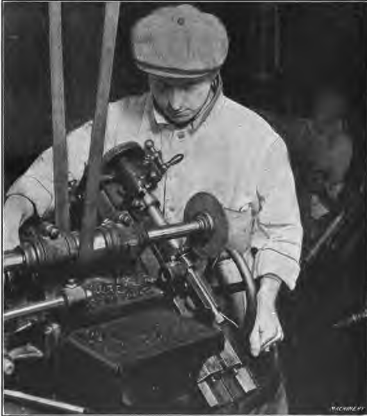
Fig. 14. Re-cutting Milling Cutters in Brown & Sharpe No. 3 Cutter Grinder
