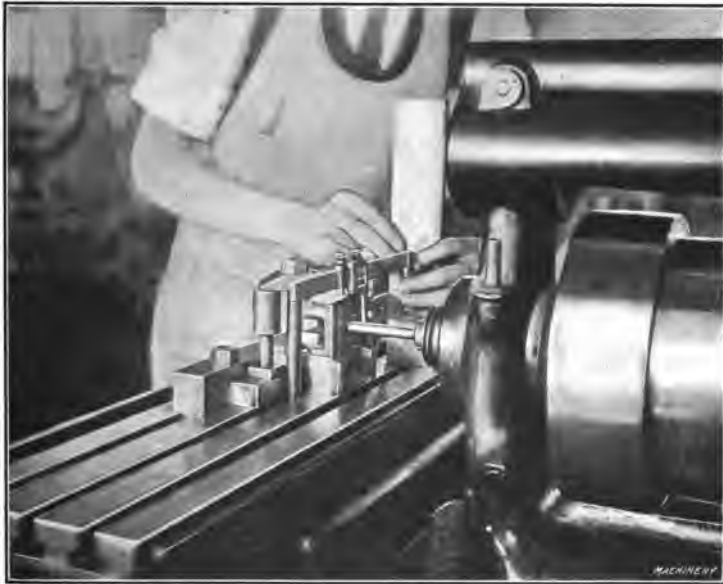
Fig. 26. Making a Horizontal Adjustment by Measuring from Angle Plate to Ground Plug
